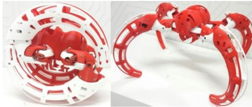
Figure 7.3 Crawling and Rolling morphologies of our Scorpio robot
