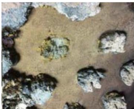
(a) Expanded bentonite status inside of liner
