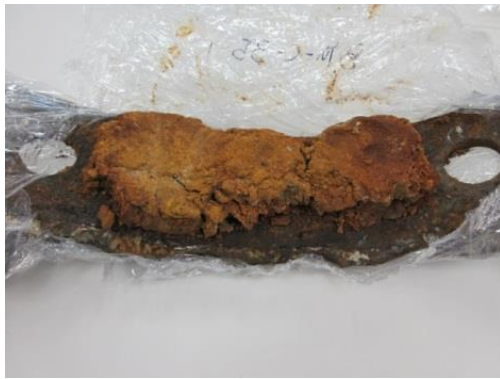
(a) Bentonite status after saturation
