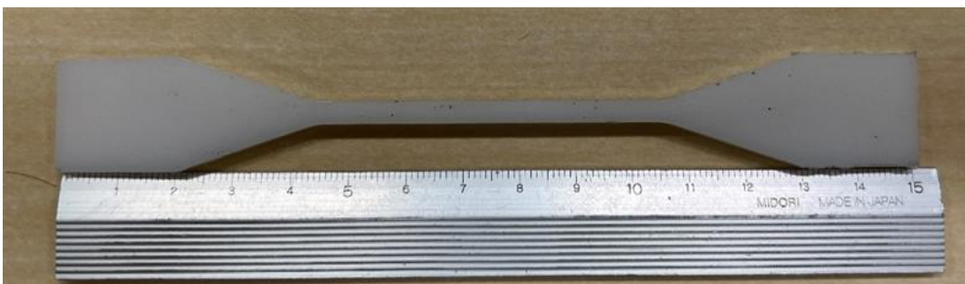
Fig. 4.6. Dumbbell-shaped test piece made of PE.
