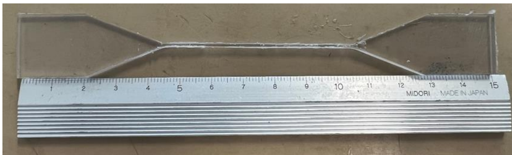
Fig. 4.8. Dumbbell-shaped test piece made of PET.
