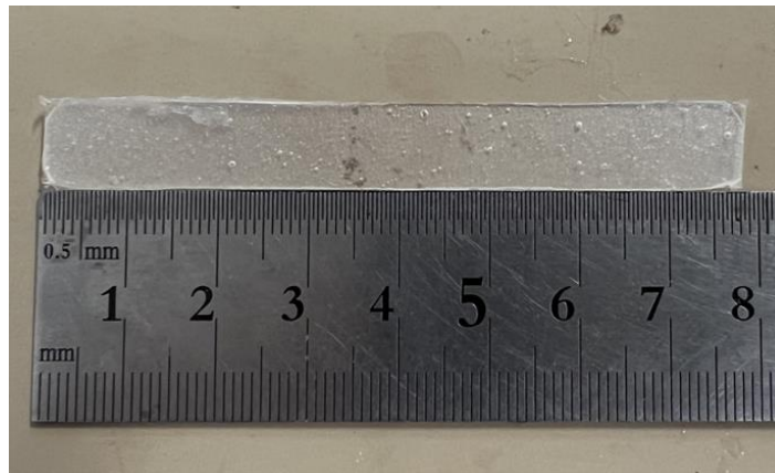
Fig. 4.9. Epoxy resin made test piece for Young's modulus measurement
