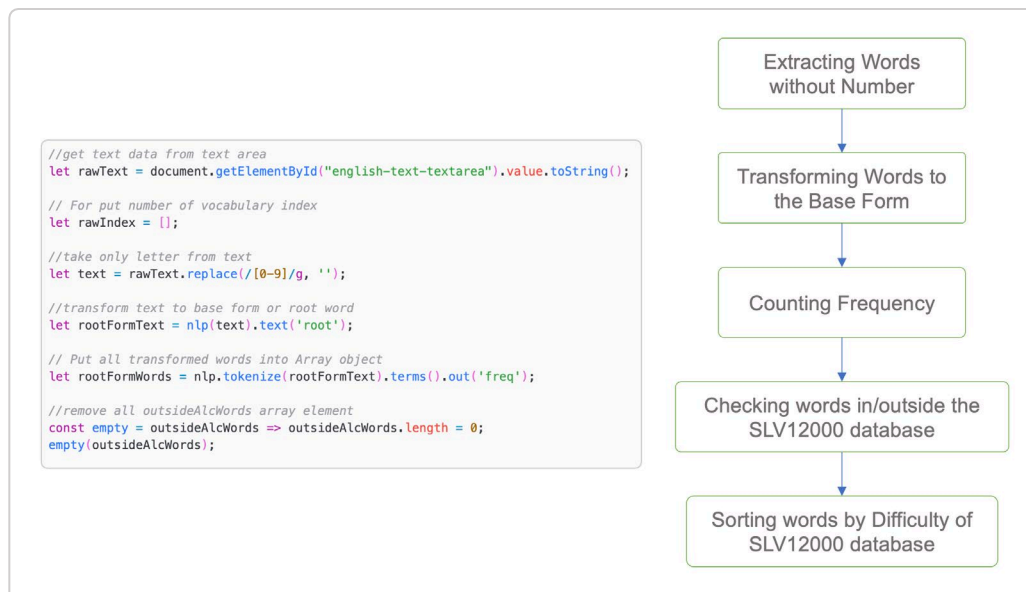
Figure 29 Morphological Analysis Function was Divided into 5 Stages
