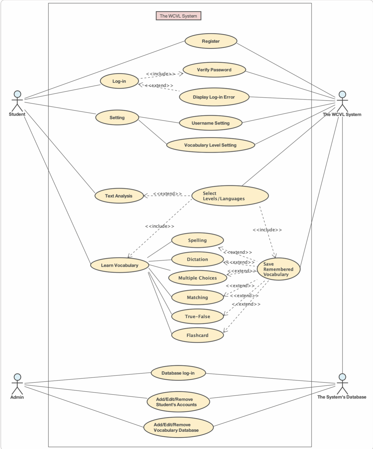
Figure 7 The High-Level Use Case Diagram of the WCVL system
