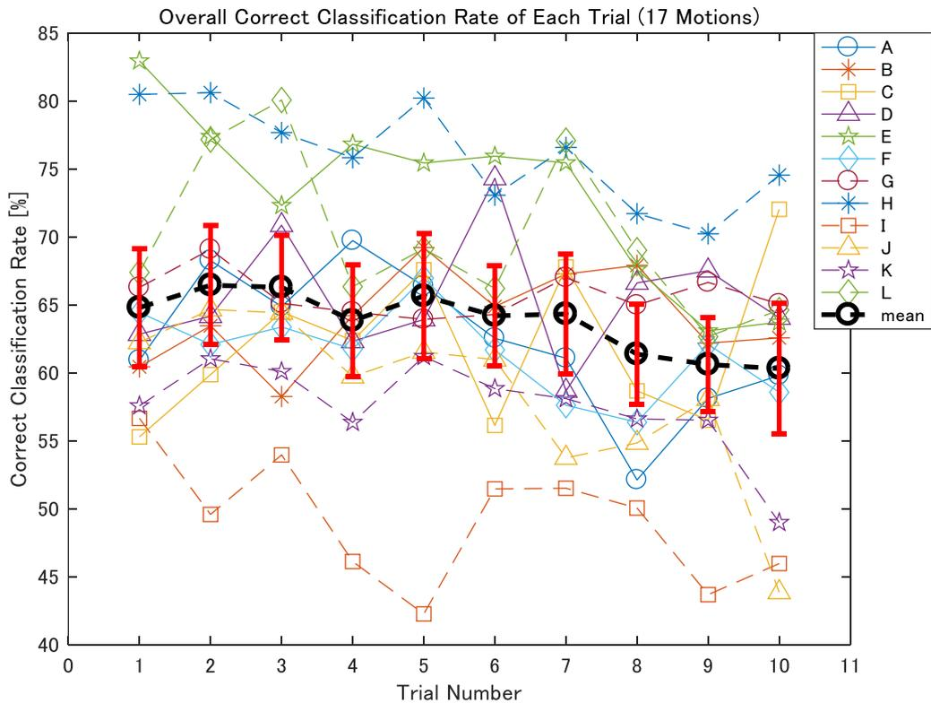
Fig. 5.12 Correct classification rate of 17 voluntary movements of each trial. Note that the correct rates of participant A, B, E and H are from the experiment on day 2 (best classification).
