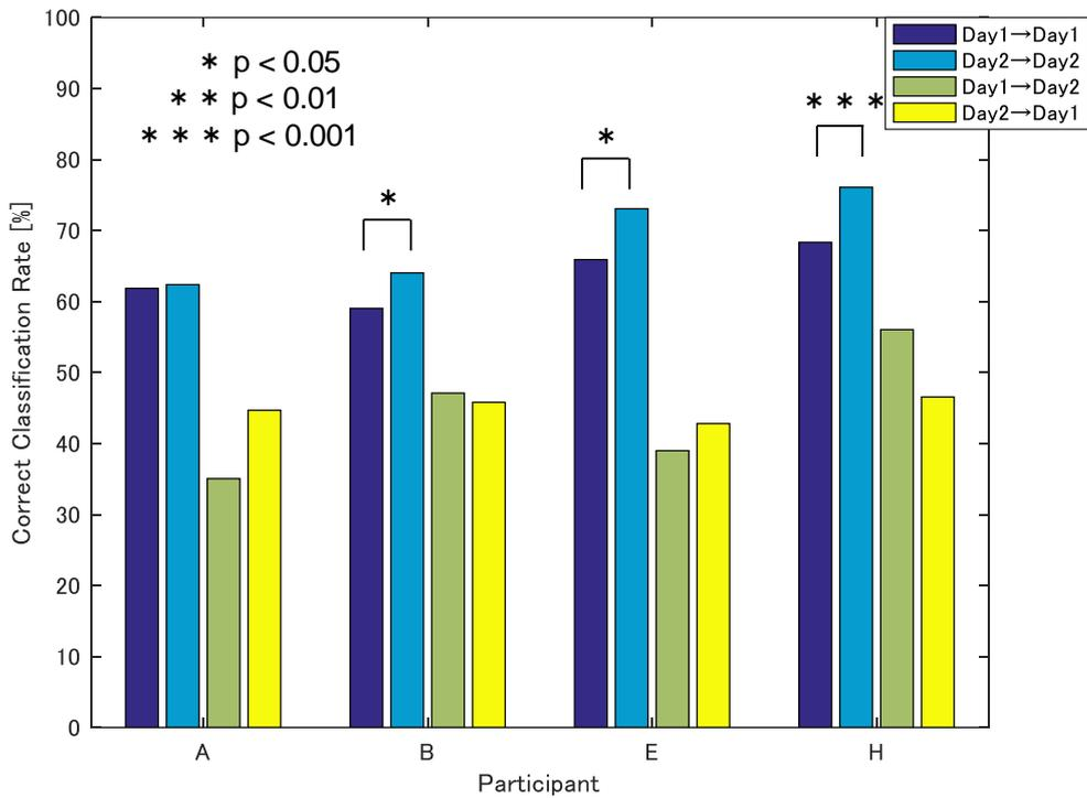
Fig. 5.11 Comparison of mean correct rates of each classification scenario (17 Movements). (\*) represents  $p < 0.05$  and (\*\*\*) represents  $p < 0.001$ .
