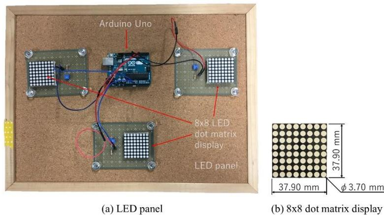
Fig. 3.3 View of the LED panel: (a) Three 8x8 dot matrix displays are used to elicit SSVEP response. The Arduino is programmed to modulate the blinking frequencies; (b) Dimensions of the dot matrix display.
