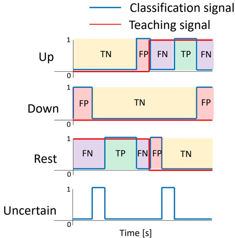
Fig. 4.11 Classification signal during up imagery task trial. From the top, classification signal of up intention, down intention, rest state and uncertain state. At each sampling time, the classification signal can take one of the following states: up, down, rest and uncertain.
