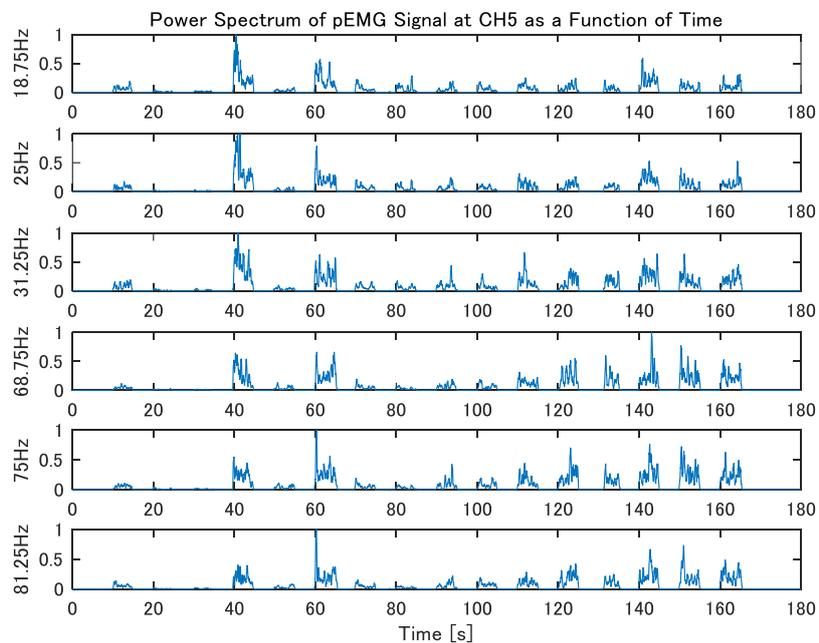
Fig. 5.7 An example of PSDs prior to log transform of 17 motions shown as a function of time. The PSDs are derived from pEMG signals on channel 5. In order from the top, PSDs at 18.75 Hz, 25 Hz, 31.25 Hz, 68.75 Hz, 75 Hz, 81.25 Hz. Note that the PSDs are normalized for better visualization.
