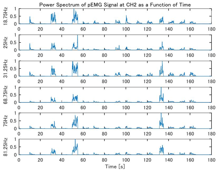
Fig. 5.6 An example of PSDs prior to log transform of 17 motions shown as a function of time. The PSDs are derived from pEMG signals on channel 2. In order from the top, PSDs at 18.75 Hz, 25 Hz, 31.25 Hz, 68.75 Hz, 75 Hz, 81.25 Hz. Note that the PSDs are normalized for better visualization.
