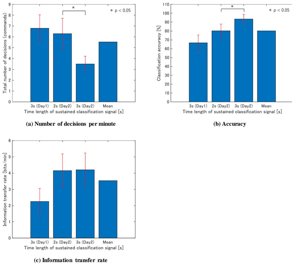
Fig. 3.12 Information transfer capability of participant B: (a) The number of decision (commands per minute); (b) Accuracy of 10 trials; (c) Information transfer rate (ITR). In all three subfigures, red error bars indicate standard deviation. (\*) represents  $p < 0.05$ .
