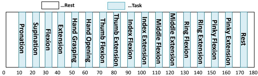
Fig. 5.8 Execution sequence of 17 motions (including rest state). Each motion is executed for five seconds with a five second resting interval in between each motion. The total duration of each run is 180 seconds. The feature point for rest state is selected between 170 to 175 seconds.
