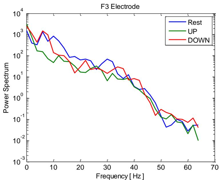
Fig. 4.8 Spectral power at F3 electrode shown as a function of frequency. In this figure, the spectral power for rest state and up imagery task is calculated by performing FFT on the EEG signals of Fig. 5 at 24 seconds and 67 seconds, respectively. Similarly, spectral power for down imagery task is calculated by performing FFT on the EEG signals of Fig. 6 at 68 seconds
