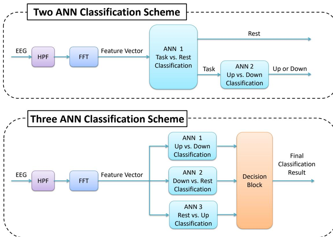
Fig. 4.13 Classification scheme using multiple artificial neural networks.
