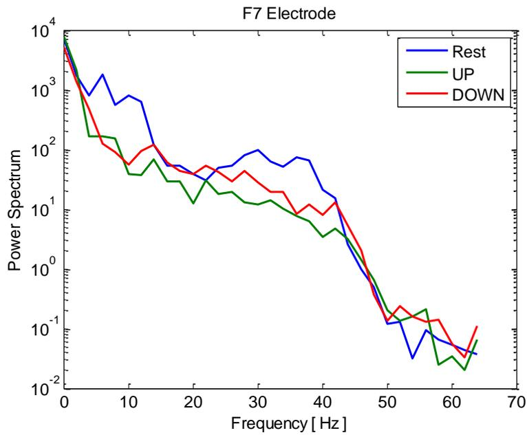
Fig. 4.7 Spectral power of F7 electrode shown as a function of frequency. In this figure, the spectral power for rest state and up imagery task is calculated by performing FFT on the EEG signals of Fig. 5 at 24 seconds and 67 seconds, respectively. Similarly, spectral power for down imagery task is calculated by performing FFT on the EEG signals of Fig. 6 at 68 seconds
