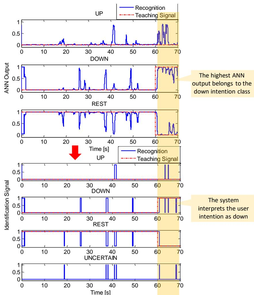
Fig. 4.10 An example of the generation of identification signals (classification of 3 mental states). The top three rows corresponds to the ANN output signal of up intention, down intention and rest state. The last four rows corresponds to the identification signal of up intention, down intention, rest state and uncertain state. At each sampling time, the ANN output signal can take one of the following states: up, down and rest. Similarly, the
