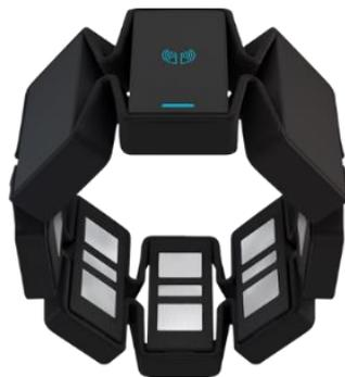
Fig. 6.3 Myo armband. 8 electrodes for EMG recording are arranged in a circular array. The sensor is also equipped with a 9-axis IMU. The EMG data is acquired at 200Hz while the IMU data is acquired at 50Hz.
