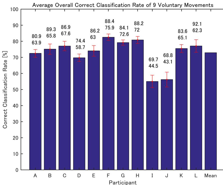
Fig. 5.13 Average overall correct classification rate of 9 voluntary movements of 12 participants. The red error bars indicate standard deviation. The two numbers on top of the bars indicate highest and lowest overall correct rate. Note that the average correct rate of participant A, B, E and H are from the experiment on day 2 (best classification). Also, the mean overall correct rate indicates the overall correct rate across subjects.
