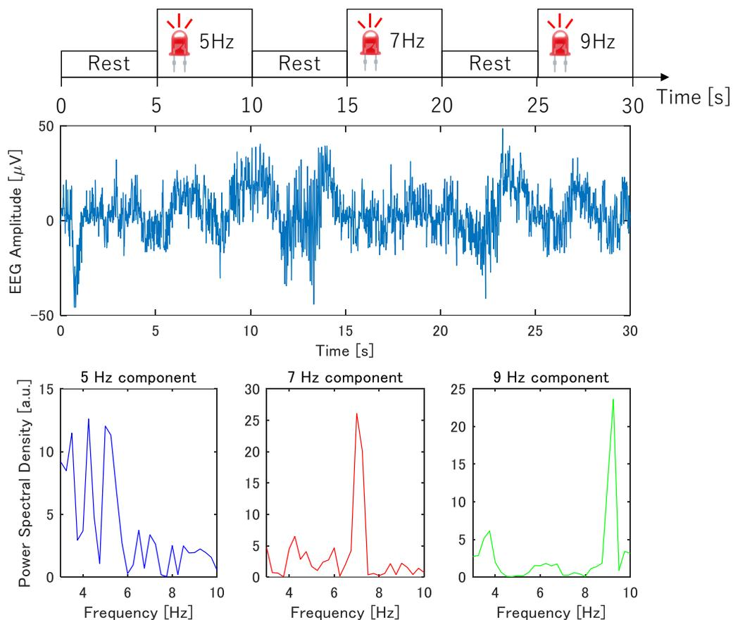
Fig. 3.1 Example of a time response of electroencephalographic signals (top subfigure) and its power spectrums while gazing at three LEDs flickering at different frequencies (lower three subfigures).
