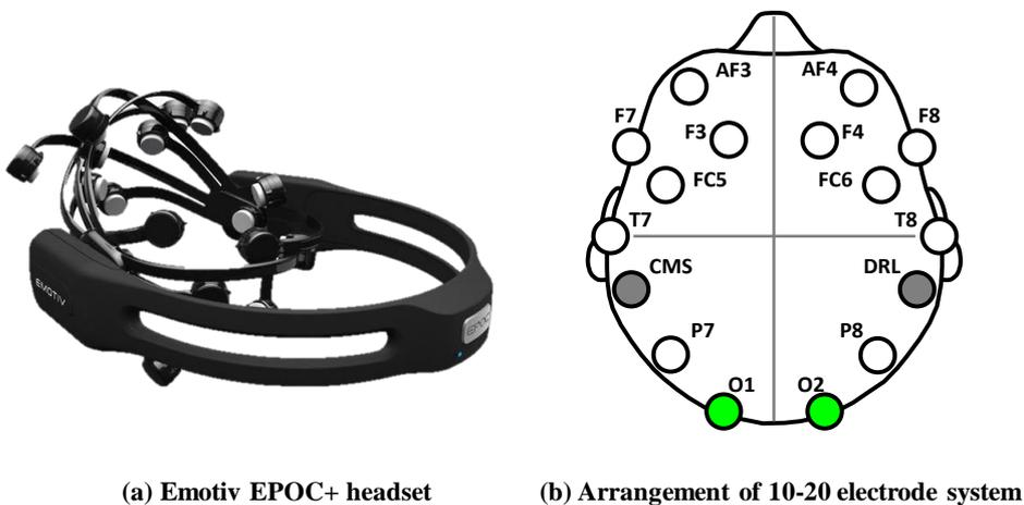
Fig. 3.7 The EEG acquisition device and the electrode arrangement: (a) The Emotiv EPOC+ headset [105]; (b) Positioning of the electrode based on the international 10-20 system. Two green circles (O1 and O2) indicate the electrodes used in this study. Two grey circles indicate the reference electrodes. Two circles highlighted in dark grey indicate reference electrodes which are located behind the ears.
