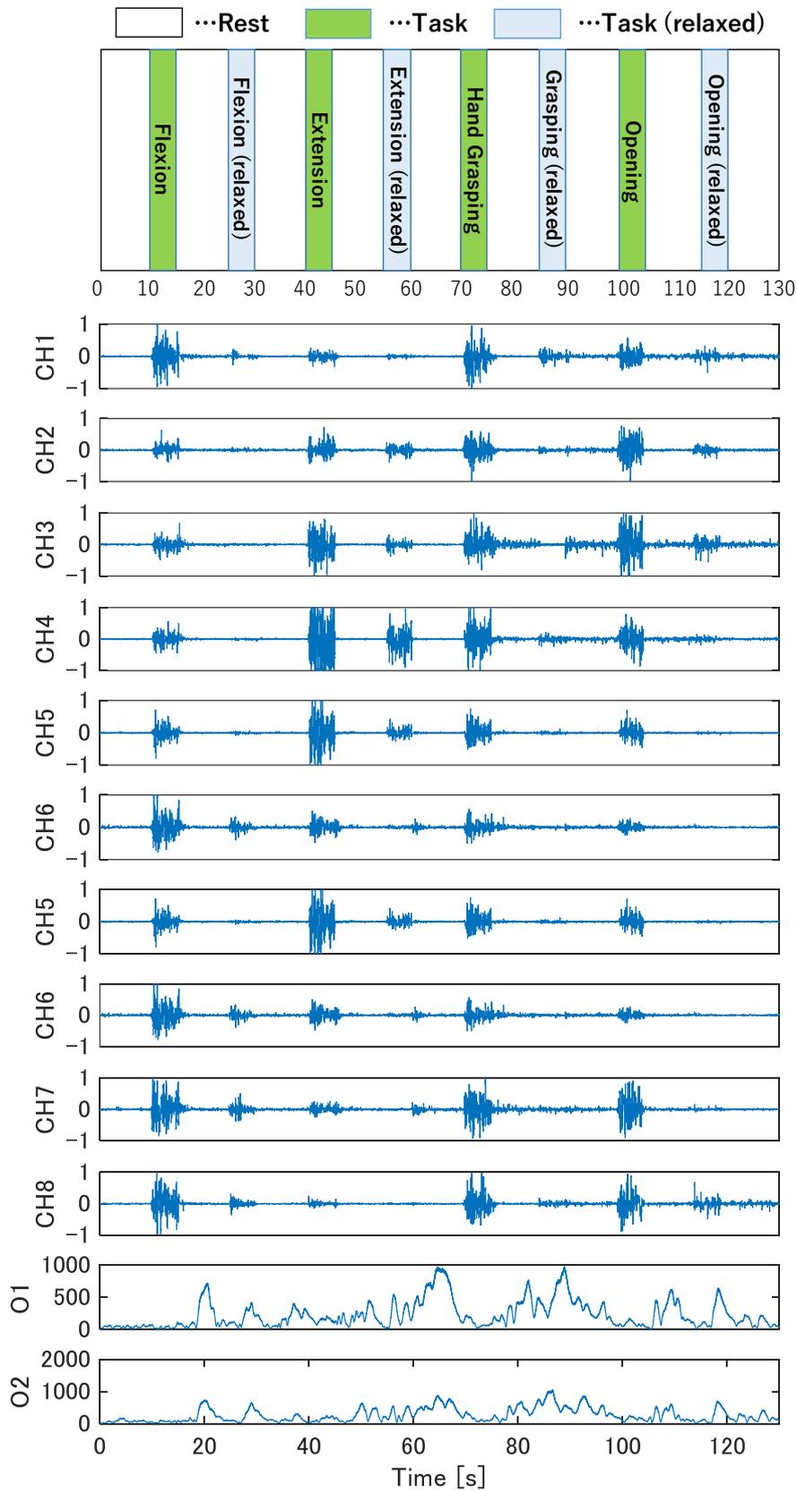
Fig. 6.6 An example of preprocessed EMG and EEG signals. The first 8 rows show the time response of preprocessed EMG signal. The last 2 rows show the time response of preprocessed EEG signal of O1 and O2 electrodes.
