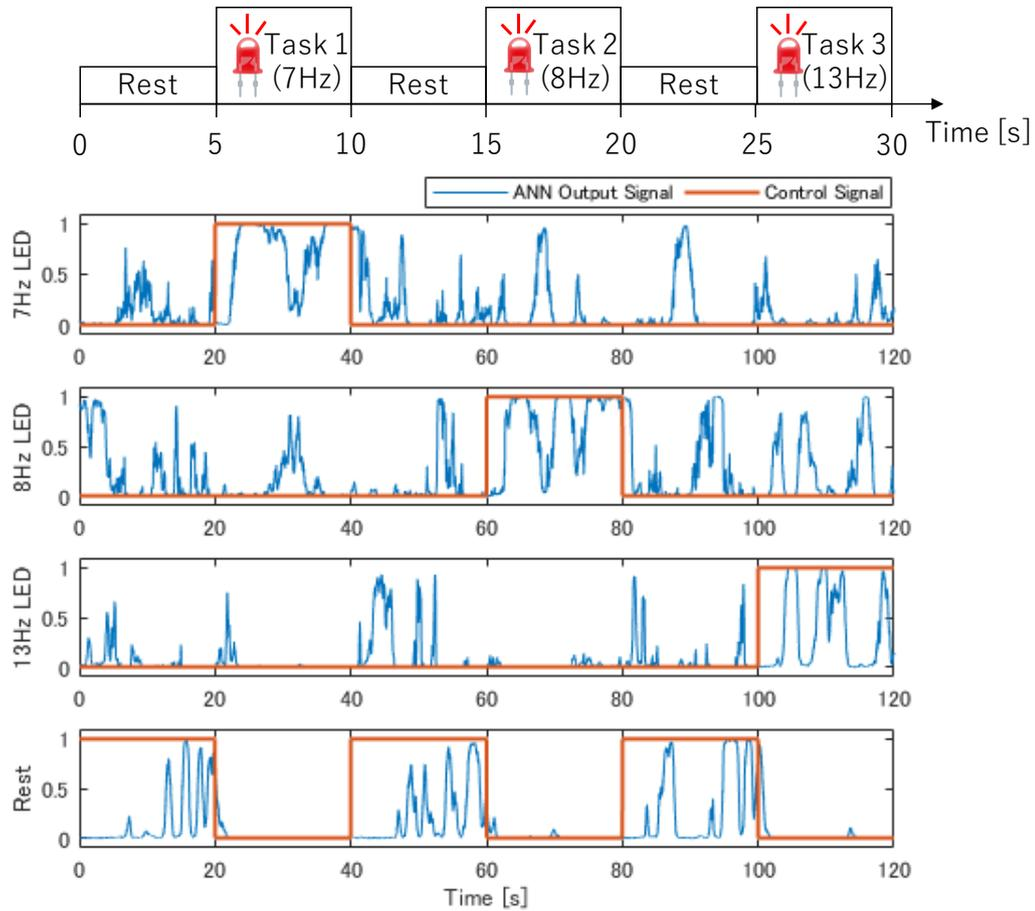
Fig. 3.9 Time responses of ANN output of participant B. From the top, output neurons corresponding to 7Hz, 8Hz, 13Hz class and rest state (in order from the top) of participant B. Leave-one-out cross-validation is performed and the result of the 3<sup>rd</sup> iteration is shown as an example. The blue line represents the classification signal. The red line represents the control signal.
