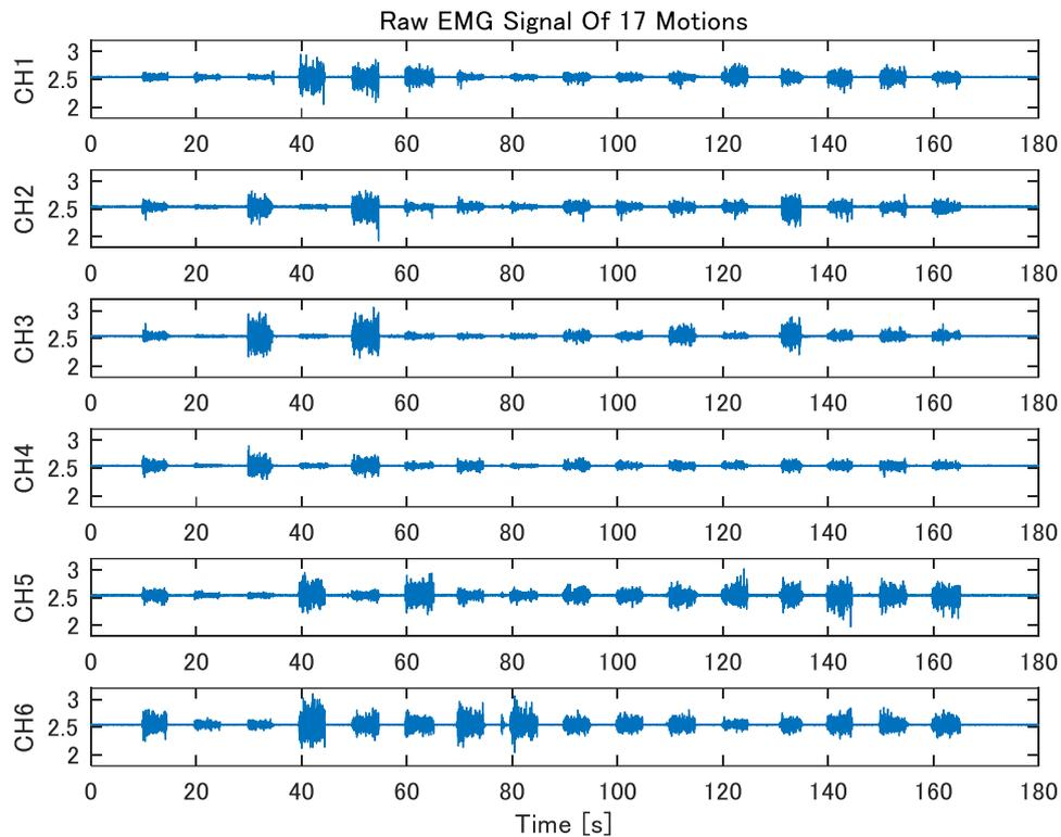
Fig. 5.5 An example of raw EMG (rEMG) signal during the execution of 17 motions. The channels are layout in ascending order starting from the top.
