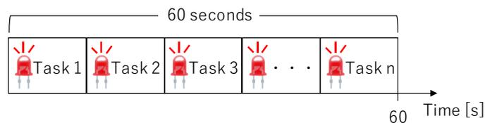
Fig. 3.6 Experimental protocol for evaluating the number of commands the BMI system can issue within one minute.
