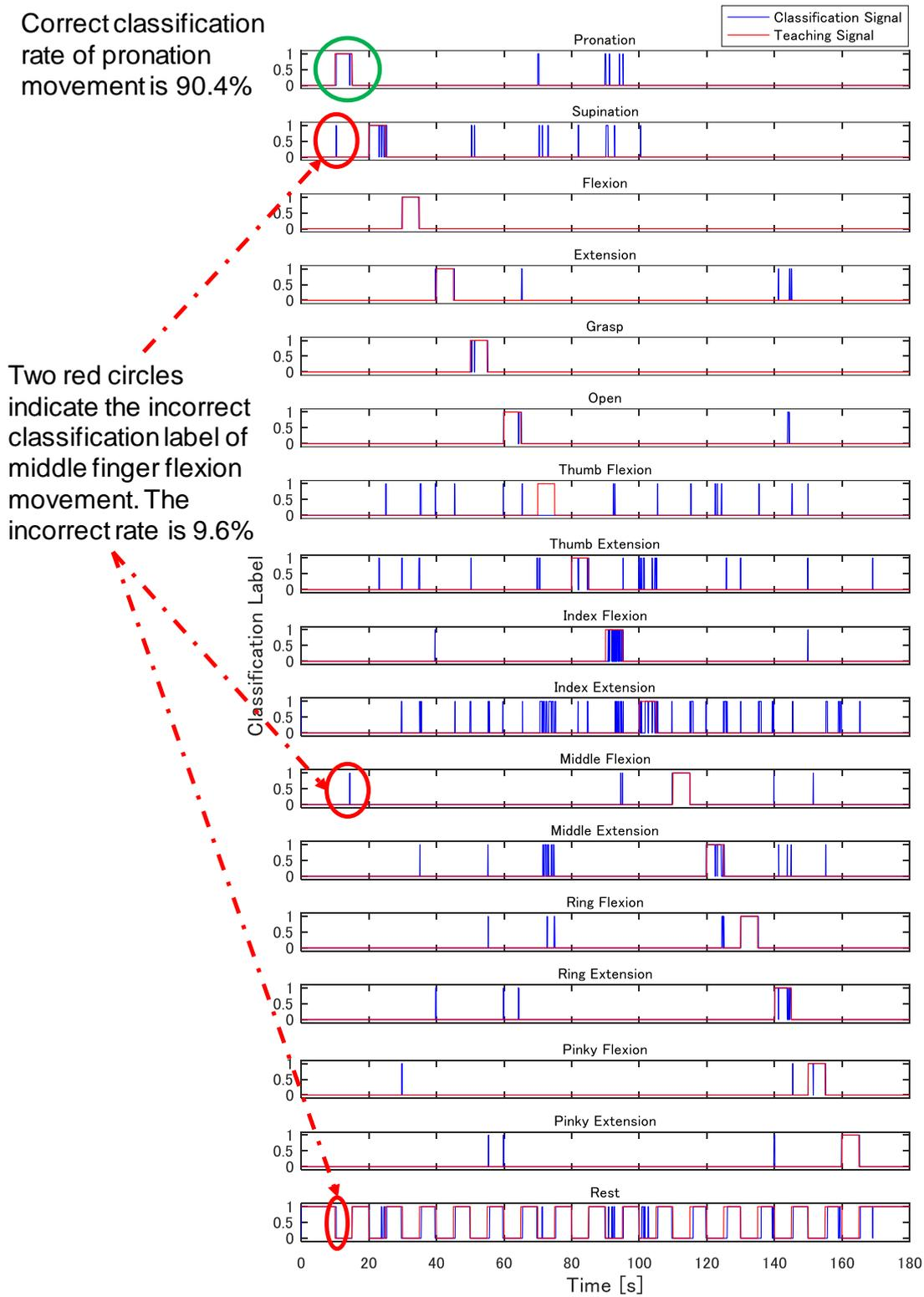
Fig. 5.9 Example of a classification output. The blue line indicates the classification signal. The red line indicates teaching signals. The green circle represents correct classification label of pronation movement as an example. The red circle indicates the incorrect classification label of pronation movement. In this study, the ANN classifier gives a decision every 0.005 seconds (200 Hz).
