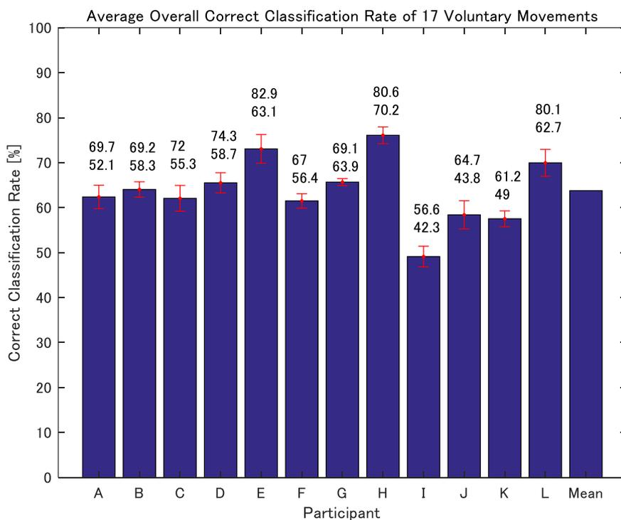
Fig. 5.10 Average overall correct classification rate of 17 voluntary movements of 12 participants. The red error bars indicate standard deviation. The two numbers on top of the bars indicate highest and lowest overall correct rate. Note that the average correct rate of participant A, B, E and H are from the experiment on day 2 (best classification). Also, the mean overall correct rate indicates the overall correct rate across subjects.
