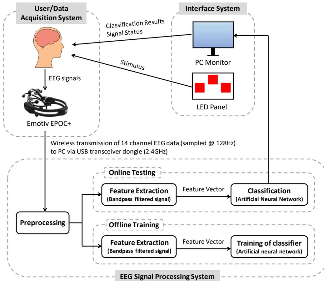
Fig. 3.2 SSVEP-based BMI system architecture
