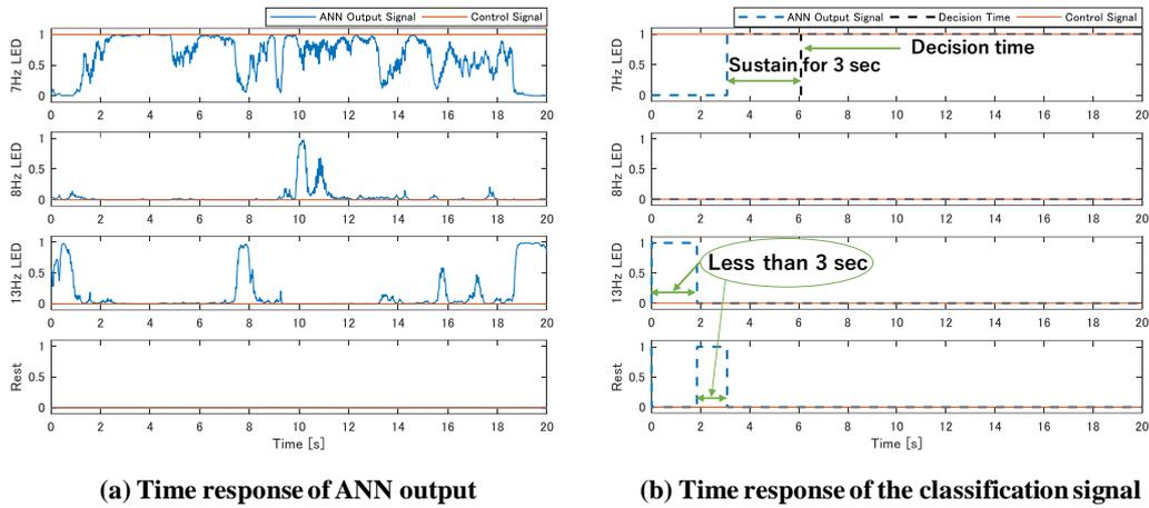
Fig. 3.10 Diagram illustrating the definition of decision time (recognition speed): (a) Time response of ANN output of the experiment in Fig. 3.5; (b) Time response of the classification signal derive from Fig. 3.10(a). In this example, the recognition speed of 7Hz LED stimulus is 6.09 seconds.
