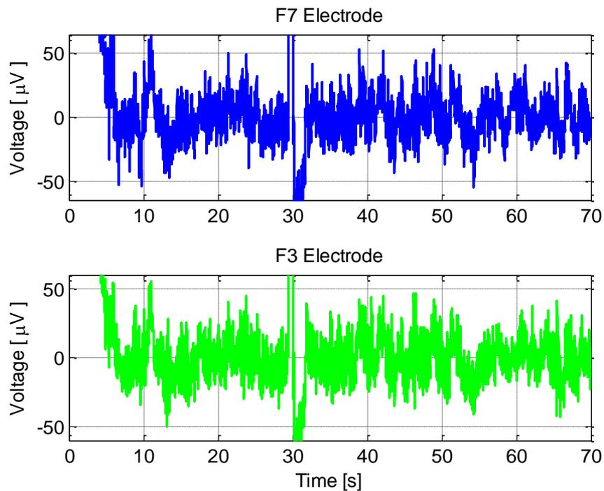
Fig. 4.6 Electroencephalograph signals during down imagery task at F7 and F8 electrode. The experiment starts with a 60 seconds rest period followed by a 10 second MI task
