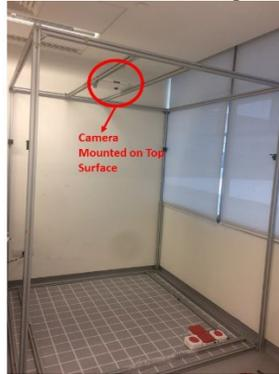
Figure 4.12. Test area with parallelepiped structure with provision for camera mount
