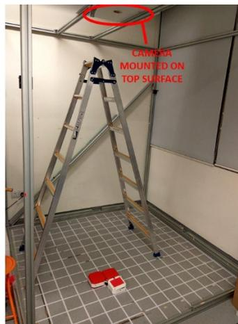
Figure 5.15. Test area with parallelepiped structure with provision for camera mount
