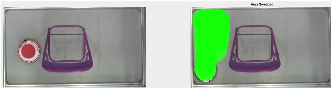
(a) Vision based benchmarking scheme for processing video with the circular-shaped robot.
